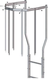
Assemble the safety cage set using M10x20 bolts and nuts. Adjust the safety cage hoops horizontally.
