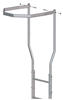
If a safety cage is needed, start at the top and install the safety cage hoops against the inside of the handrail. The hoops can be widened by hand for the best fit.
